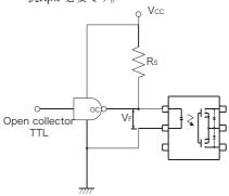
Another example circuit that can be used with open-collector TTL gate is shown the following figure. This driving circuit eliminates the extra pull-up resistor, Rp, required by the circuit in above figure.
