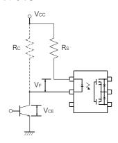
$$Rs = \frac{V_{CC} - V_{CE(sat)} - V_F}{I_F}$$
