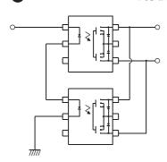
In principle, it should be avoided to use relays in parallel to increase the current capacity. When using them in parallel, do not exceed the absolute maximum rating of the load current for each relay. However the usage in parallel is effective to reduce On-Resistance.
