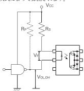
$$Rs = \frac{V_{CC} - V_{OL} - V_{F}}{I_{F}}$$
